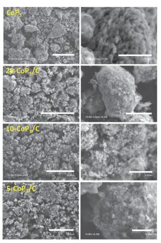
Fig. 4 Representative SEM images of  $CoP_3$  and  $x-CoP_3/C$  (x = 5, 10, 25 mol%) powders from reactions of x-CoCl<sub>2</sub>/C and red phosphorus at 500 °C. Scale bars are 50 μm for all left images. Scale bar lengths for right images of CoP<sub>3</sub> and 10-CoP<sub>3</sub>/C are 5  $\mu$ m and 25-CoP<sub>3</sub>/C and 5-CoP<sub>3</sub>/C are 10 μm
