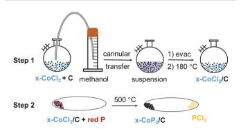
Fig. 1 Schematic of two-step synthesis procedure of x-CoP<sub>3</sub>/C (x = 5, 10, 25 mol%) materials. Step 1 shows methanol precipitation of CoCl<sub>2</sub> onto C (XC-72 carbon black), and step 2 shows direct reaction of x-CoCl<sub>2</sub>/C with elemental red phosphorus at 500 °C.
