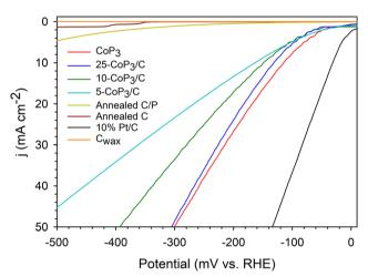
Fig. 6 Representative LSV data for x-CoP<sub>3</sub>/C (x = 5,10, 25 mol%) powders on C<sub>wax</sub> electrodes using Pt counter and SCE reference electrodes in 0.5 M H<sub>2</sub>SO<sub>4</sub> (5 mV s<sup>-1</sup> scan rate, no iR compensation) in a three-electrode cell. An LSV overlay graph with 85% iR compensated data is shown in Fig. S15 (ESI†). Plots for C<sub>wax</sub>, annealed C, annealed C/P and commercial 10% Pt/C are shown for comparison.
