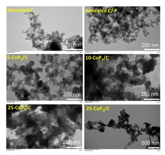
Representative TEM images of x-CoP<sub>3</sub>/C (x = 5, 10, 25 mol%) particles and aggregates synthesized from direct reactions of x-CoCl<sub>2</sub>/C (x = 5, 10, 25 mol%) with elemental red phosphorus at 500 °C.
