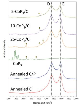
Fig. 3 An overlay of Raman spectra of  $CoP_3$ ,  $x-CoP_3/C$  (x = 5,10, 25) and 500 °C annealed carbon black alone (C) and carbon black annealed with phosphorus (C/P) in the region of 200–2000 cm<sup>-1</sup>. ( $\diamondsuit$  denotes peaks for P–O bonding).
