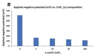
Fig. 7 (A) Comparison of trends of physical BET surface area and electro-25 mol%) materials along with annealed C/P (x = 0). (B) Variation of applied negative potentials (iR uncompensated) to achieve a 10 mA cm<sup>-2</sup> current density with the amount of CoP<sub>3</sub> dispersed on carbon black composites.
