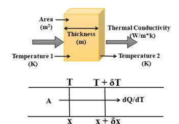
Fig. 7 A typical heat flow mechanism inside the conductor.
