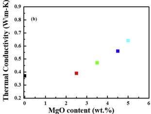
Fig. 20 Experimental data showing the thermal conductivity of NaNO $_3$ -KNO $_3$  (a) improves with the addition of MgO at different mass concentrations (2.5%, 3.5%, 4.5% and 5%) with temperature, and (b) the increasing thermal conductivity at different concentrations. Adapted from ref. 35, with permission from Elsevier, Copyright 2020.
