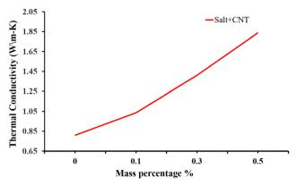
Fig. 22 Experimental data showing how the thermal conductivity of NaNO<sub>3</sub>-KNO<sub>3</sub> improves with addition of CNT at different mass concentrations of 0.1%, 0.3% and 0.5%. Adapted from ref. 39, with permission from the American Chemical Society, Copyright 2023
