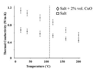
Fig. 18 Experimental data showing elevation in thermal conductivity before and after addition of CuO nanoparticles to  $NaNO_3$ - $KNO_3$ . Adapted from ref. 34, with permission from Elsevier, Copyright 2016.
