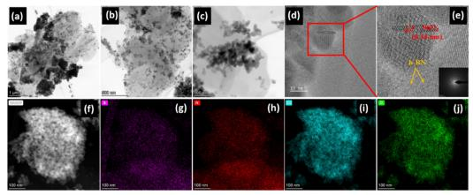
Fig. 3 (a-c) TEM images of  $SnO_2/10\%$  h-BN, (d) HRTEM image, and (e) SAED of  $SnO_2/10\%$  h-BN (bright field); (f) TEM image and the corresponding (g) boron, (h) nitrogen, (i) tin, and (j) oxygen EDX elemental mappings of a  $SnO_2/10\%$  h-BN particle.
