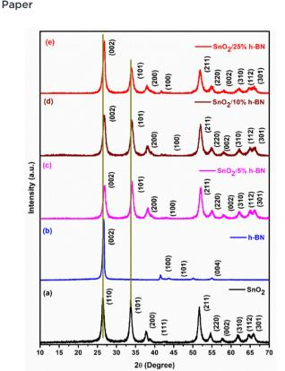
Fig. 1 XRD patterns of (a)  $SnO_2$ , (b) h-BN, (c)  $SnO_2/5\%$  h-BN, (d)  $SnO_2/5\%$ 10% h-BN and (e) SnO<sub>2</sub>/25% h-BN composites
