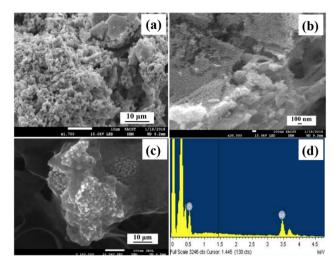
Fig. 2 (a) and (b) SEM images of pure SnO<sub>2</sub>, (c) SEM and (d) EDX of the SnO<sub>2</sub>/10% h-BN nanocomposite.
