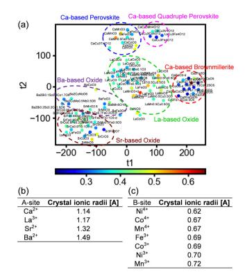
Fig. 3 Data distribution obtained using t-SNE analysis including single Asite-containing multimetal oxides. The plot colors indicate the overpotential of each catalyst. (b) and (c) Ionic radii for the typical A-site and Bsite metals, respectively.34
