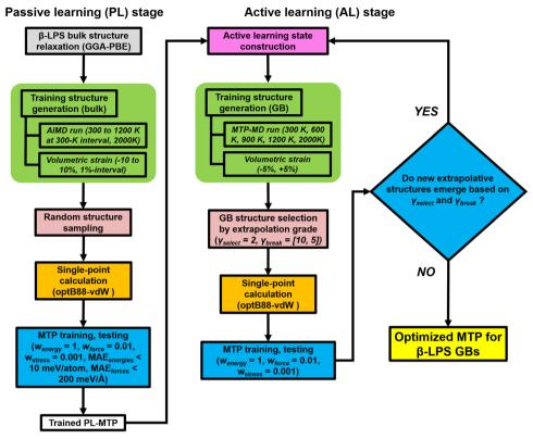
Fig. 2 Schematic workflow for passive and active learning related to MTP development for β-LPS GBs.
