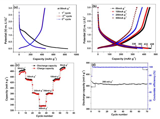
Fig. 5 Galvanostatic charge discharge profiles of CNTs on the Cu substrate. (a) First three charge-discharge cycles at 50 mA  $g^{-1}$ . (b) Electrode subjected to various current densities from 50-500 mA  $g^{-1}$ . (c) High-rate cycling performance. (d) Discharge capacity and coulombic efficiency vs. cycle number at the current density of 200 mA g<sup>-1</sup>.
