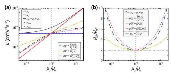
Fig. 2 (a) Different definitions of the effective mobility  $\mu_{\text{eff}}$  and photoconductance mobility  $\mu_{\text{ph}}$  as well as (b) the resulting ratio  $\mu_{\text{ph}}/\mu_{\text{eff}}$  in relation to the ratio of the hole and electron mobility  $\mu_p/\mu_p$
