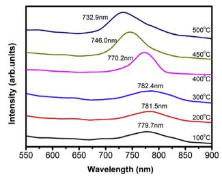
Fig. 12 Photoluminescence spectra of CdZnTe thin films deposited at varied substrate temperatures. Reproduced from ref. 79 with permission, Copyright (2016), Elsevier
