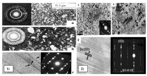
Fig. 9 TEM images of (1) Cd<sub>0.48</sub>Zn<sub>0.52</sub>Te thin films: (a) as-deposited state, (b) after in situ annealing for 15 min at 250 °C, and (c) HRTEM images. (2) In situ Cd<sub>0.48</sub>Zn<sub>0.52</sub>Te thin films annealed at 250 °C for (a) 30 min and (b) 33 min and (c) HRTEM images. Reproduced from ref. 89 with permission, Copyright (2002), Wiley-VCH
