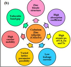
Fig. 2 (a) Crystal structure and (b) properties of CdZnTe material
