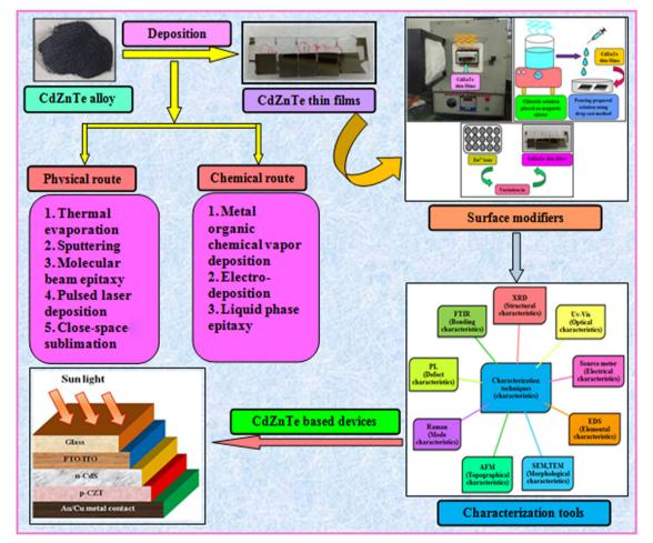
Fig. 1 Pictorial illustration of the various experimental tools used for the deposition and characterization of CdZnTe thin films, surface modifiers and the CdZnTe-based solar cell device architecture.
