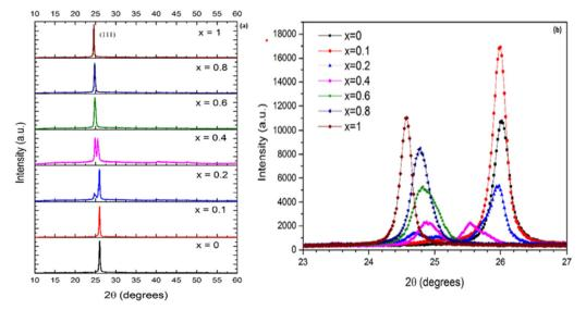
Fig. 6 (a) XRD patterns of  $Cd_{1-x}Zn_xTe$  thin films at varying Zn concentrations and (b) enlarged portion of the diffractograms in  $2\theta$  range of  $23-27^\circ$ , showing the position of the dominant peak. Reproduced from ref. 119 with permission, Copyright (2020), Elsevier Ltd.
