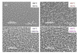
Fig. 8 Surface morphological images of (a) A1, (b) A2, (c) B1 and (d) B2 CdZnTe samples. Adapted with permission from ref. 76 Copyright (2018),
