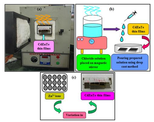
Fig. 4 Pictorial illustration of (a) thermal annealing, (b) chloride activation treatment and (c) variation in Zn content on CdZnTe thin films.
