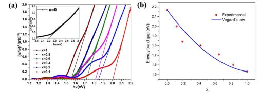
Fig. 7 (a) Tauc plots where vertical scale bears unit  $(cm^{-1} eV)^2$  and (b) variation in optical energy band gap as a function of Zn content for  $Cd_{1-x}Zn_xTe^{-x}$ thin films. Reprinted from ref. 119 with permission, Copyright (2020), Elsevier Ltd
