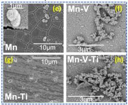
Fig. 11 SEM images of electrodeposited MnO<sub>2</sub> on the carbon felt electrodes (a)-(d) and on the glassy carbon electrodes (e)-(h), respectively (reproduced from ref. 74 with permission from Wiley-VCH).
