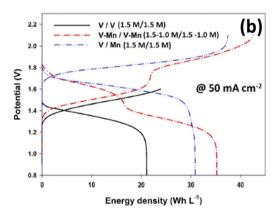
Fig. 10 (a) Photographic images of  $MnO_2$  deposition in the V/Mn and V-Mn/V-Mn system and (b) GCD profile recorded at 50 mA cm<sup>-2</sup> (reproduced from ref. 72 with permission from Elsevier).
