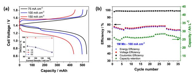
Fig. 7 (a) Galvanic charge discharge performance recorded at different current densities, and (b) H–Mn flow battery performance at 100 mA cm $^{-2}$ ; electrolyte: 1 M MnSO<sub>4</sub> + 3 M H<sub>2</sub>SO<sub>4</sub> + 1 M Ti(SO<sub>4</sub>)<sub>2</sub>, Hydrogen: 100 mL min $^{-1}$ , Flow rate: 50 mL min $^{-1}$ , respectively.<sup>55</sup>
