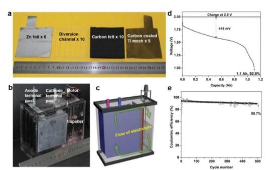
Fig. 15 (a) The cell components used for the membrane free aqueous Zn/MnO<sub>2</sub> RFB, (b) photographic image of the Zn/MnO<sub>2</sub> RFB, (c) schematic diagram of the indication of electrolyte flow, (d) the GCD profile of the Zn/MnO<sub>2</sub> RFB, and (e) the cyclability of the Zn/MnO<sub>2</sub> RFB (reproduced from ref. 87 with permission from Wiley).
