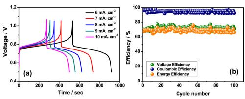
Fig. 8 (a) The GCD performance recorded at different current densities and (b) the cyclability profile of Fe/Mn RFB (reproduced from ref. 63 with permission from Elsevier).
