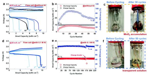
Fig. 13 The GCD performance of Zn/Mn RFB recorded at 20 mA cm<sup>-2</sup> (a)-(c) without KI and (d)-(f) with 0.1 M KI (reproduced from ref. 82 with permission from The Royal Society of Chemistry).
