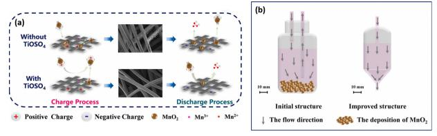
Fig. 6 Schematic illustration of (a) the TiOSO<sub>4</sub> additive in the V-Mn flow battery and (b) the improved electrolyte tank structure (reproduced from ref. 46 with permission from Elsevier)
