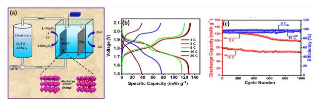
Fig. 14 (a) Schematic illustration of the single flow  $Zn/\lambda-MnO_2$  RFB, (b) the GCD profile of single flow  $Zn/\lambda-MnO_2$  RFB at different C rates, and (c) long cycling performance of Zn/ $\lambda$ -MnO<sub>2</sub> RFB recorded at 2 and 10C rates.<sup>86</sup>
