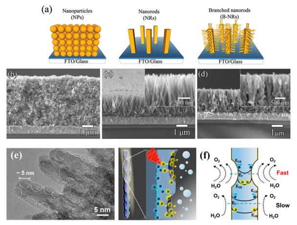
Fig. 5 (a) Schematic diagram of the synthesis of  $TiO_2$  branched nanorods. SEM images of (b)  $TiO_2$  nanoparticles, (c) nanorods, and (d) branched nanorods. Reprinted with permission from ref. 43. Copyright © 2011, American Chemical Society. (e) TEM image of the TiO<sub>2</sub> nanowire arrays. (f) Schematic illustrations of the hole extraction effect of TiO<sub>2</sub> nanowire arrays. Reprinted with permission from ref. 45. Copyright © 2022, American Chemical Society.
