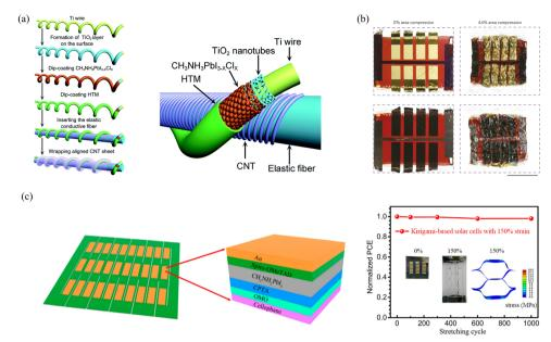
Fig. 3 (a) Schematic illustration of the elastic PSC fibre; 53 (b) schematic of the ultrathin and buckling FPSCs; 54 (c) schematic illustration of the kirigamibased PSC array and structure of PSCs and normalized PCE of kirigami-based PSCs after different stretching cycles.<sup>55</sup>
