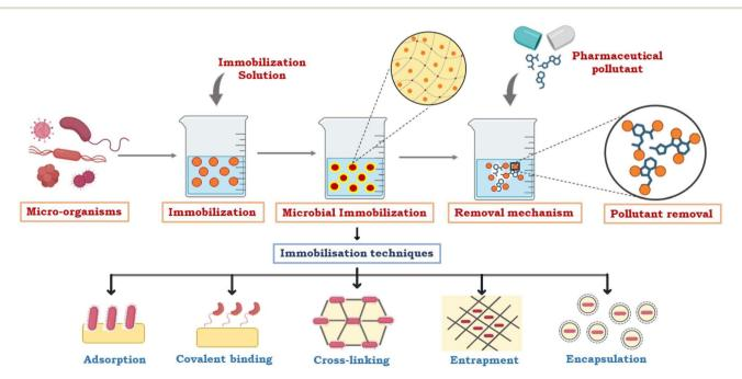
Fig. 4 Microbial immobilization for the removal of pharmaceutical pollutants.
