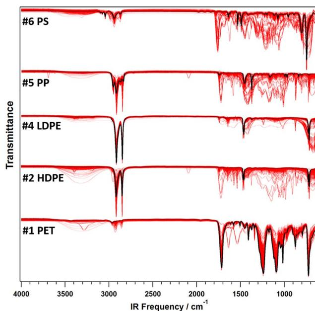
Fig. 2 Mid-infrared (4000–650  $\text{cm}^{-1}$ ) spectra of 835 postconsumer plastics that were evaluated in this study (red). Virgin polymer (black). Spectra are shown in percent transmittance ( $y$ -axis minimum is 30% per RIC).
