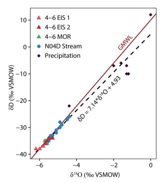
Fig. 6 Stable water isotopes in stream water, groundwater, and precipitation samples collected at N04D. Solid line denotes the global meteoric water line (GMWL) ( $\delta D = 8 \times \delta^{18}O + 10$ ), and the dashed line denotes the linear regression of all plotted samples. Isotope data are available in the ESI (Tables SI3–SI5†).
