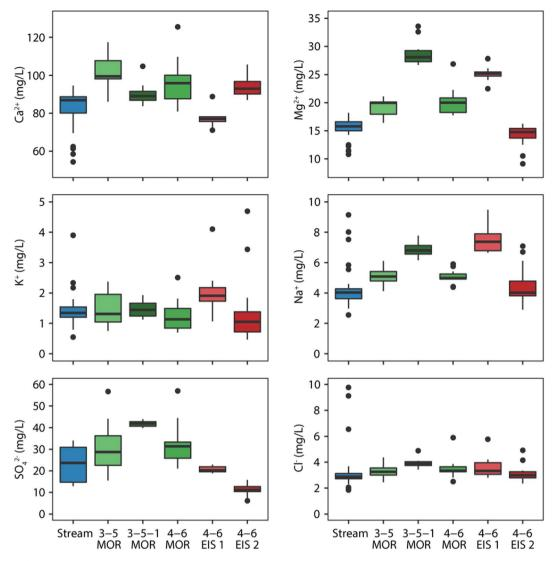
Box plots of select major ion concentrations in all surface and groundwater samples. Hinges mark the interquartile range of each group of samples, and stems extend to 1.5 times the interquartile range. Individual points mark outlier samples that had concentrations greater or less than 1.5 times the interquartile range. Extreme outlier points are not shown for  $K^+$  and  $Cl^-$  to show finer variation in concentrations. Complete data are available in the ESI (Tables SI3 and SI4†).
