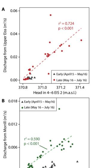
Fig. 10 Relationship between volumetric input to the stream of water from the (A) Upper Eiss Ls and (B) Morrill Ls, and head in their respective wells. Dotted regression lines are fit only to the samples collected after May 16. Grey triangles denote samples which were collected prior to May 14.
