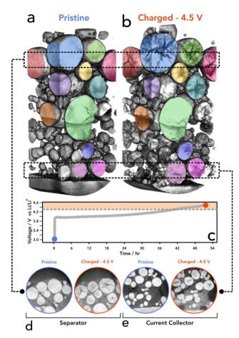
Fig. 1 (a and b) Volume rendering of the same region of an NMC811 electrode at (a) blue – pristine and (b) red – charged state (4.5 V s Li/Li<sup>+</sup>). (c) Charging profile for NMC811 electrode to 4.5 V at C/50, noting potentials at which the two nano-CT datasets were collected. (d and e) Representative ortho slices of the same particles at pristine and charged state at (d) separator and (e) current collector.
