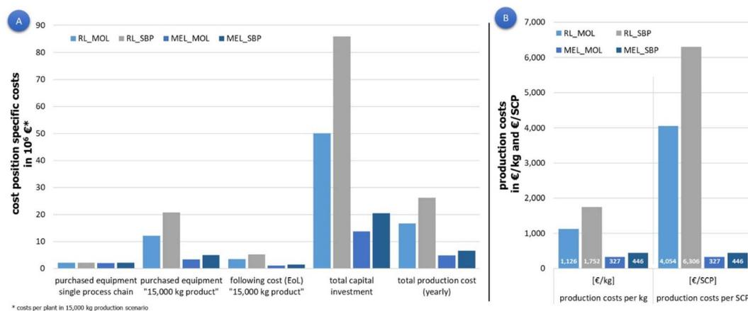
Fig. 6 Results in a 15 Mg production scenario for (A) different purchased equipment data, capital investment, yearly production cost and End-of-Life (EoL) cost for the production plant per process chain and (B) production costs per process chain expressed per kg and per SCP.
