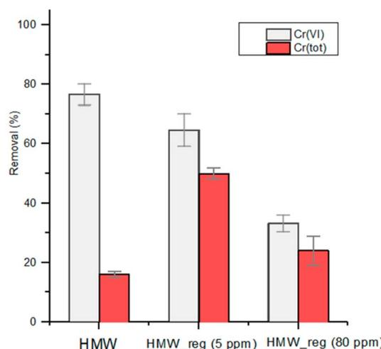
Fig. 7 Reduction of Cr(vi) by HMW and two regenerated lignins, HMW\_reg\_5 and HMW\_reg\_80. pH 2 obtained with  $2 \text{ M HNO}_3$ ;  $1 \text{ g L}^{-1}$  of lignin; initial Cr(vi) concentration:  $5 \text{ mg L}^{-1}$ ; contact time: 2 h.
