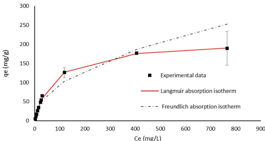
Fig. 11 Isotherm model fitting of Cr(vi) adsorption on EH lignin as the adsorbent.
