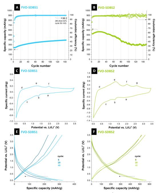
Fig. 5 (A) and (B) Stability of FVO-SDBS1 and FVO-SDBS2 at the specific current of 250 mA g<sup>-1</sup>, respectively. (C) and (D) The respective cyclic voltammetry at the scanning rate of 0.1 mV s<sup>-1</sup>, and (E) and (F) the respective galvanostatic charge-discharge curves
