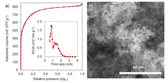
Fig. 4 (a) N<sub>2</sub> adsorption isotherm (inset: QSDFT PSD) and (b) SEM micrograph of AGA-850.
