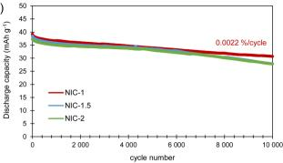
Fig. 7 (a) Ragone plot showing the energy/power performance of the NICs and (b) long-term cycling test performed at 2 A  $g^{-1}$ .
