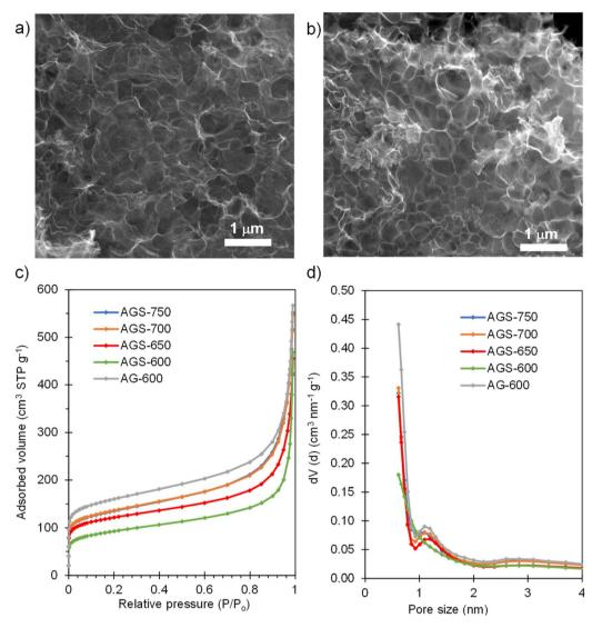
Fig. 2 SEM micrograph of (a) AGS-600 and (b) AGS-750; (c) N<sub>2</sub> adsorption isotherms and (d) pore size distributions of the non-doped material and materials doped with S at different temperatures.
