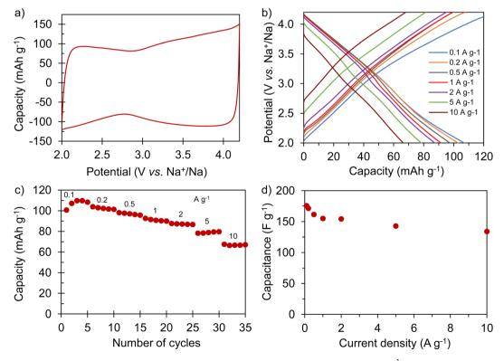
Fig. 5 Electrochemical characterization of AGA-850: (a) cyclic voltammogram recorded at 2 mV s<sup>-1</sup>; (b) galvanostatic charge-discharge potential profiles recorded at different current densities; rate capability expressed in terms of (c) capacity and (d) capacitance.
