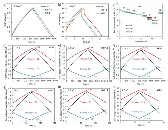
Fig. 6 Electrochemical characterization of the full cells: (a) galvanostatic charge–discharge profiles recorded at (a) 0.1 A g<sup>-1</sup> and (b) 10 A g<sup>-1</sup>; (c) evolution of capacity with the current density; (d-i) potential/voltage profiles of the full cell (black), positive electrode (red) and negative electrode (blue) of NIC-1, NIC-1.5 and NIC-2 recorded at 0.1 A g<sup>-1</sup> and 2 A g<sup>-1</sup>.
