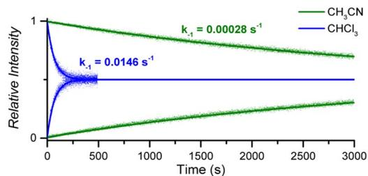
Fig. 5 Relative time evolution of  $[\text{CoC}(\text{Py}_{\text{IN}})]^+$  (top traces and lines) and  $[\text{CoC}(\text{Py}_{\text{IN}})]^+$  (bottom traces and lines) in DRL experiments carried out at 40 °C in chloroform (blue traces) and acetonitrile (green traces) in the presence of 100 equiv. pyridine and 100 equiv. pyridine-D5. Dots are experimental data points, and lines correspond to fittings of experimental data by eqn (S1) and (S2).†
