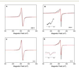
Fig. 2 Experimental (black) and simulated (red) X-band CW-EPR spectra of polycrystalline compound  ${\bf 1}$  at (A) 298 K, and (C) 10 K; and compound  ${\bf 2}$  at 298 K (B) and 10 K (D). Inset in (B) and (D) show the half-field region, with simulation in red. Parameters are provided in the text.
