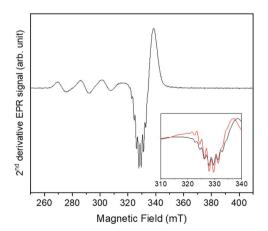
Fig. 3 Second harmonic X-band CW-EPR spectrum of compound 2 at 50 K (black) and its simulation (red). Inset shows the simulation of the  $g_{xy}$  region, evidencing hyperfine couplings with  $^{63,65}$ Cu and  $^{14}$ N.
