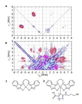
Fig. 5 Experimental (blue) and simulated (red: N1, N4; magenta:  $N_{\text{triazole}}$  (N6, N7)) X-band  $^{14}$ N HYSCORE spectra of (A) compound 1 and (B) compound 2, schematically represented below.
