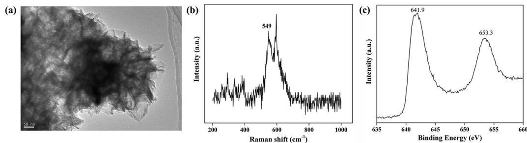
Fig. 6 (a) TEM image, (b) Raman spectrum and (c) XPS of MnO<sub>2</sub> nanosheets.
