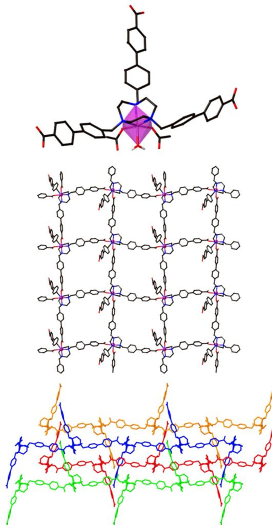
Fig. 2 Magnified view of the hexacoordinated Co node in the structure of poly-[Co<sub>2</sub>(H<sub>2</sub>)(OH<sub>2</sub>)]·2DMF·4H<sub>2</sub>O (top), simplified view of the framework viewed along the crystallographic *a*-axis (middle), and an expanded view to highlight how the sheets stack with interdigitation in the *x* direction (bottom).
