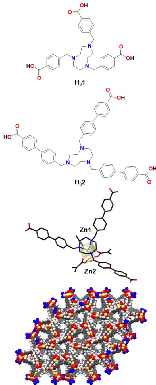
Fig. 1 Designed TACN-based tricarboxylic acid H<sub>3</sub>2 with extended, rigid arms compared to the previously reported H<sub>3</sub>1 (top), magnified view of the dinuclear Zn cluster in poly-[Zn<sub>2</sub>(2)(OH)<sub>2</sub>]Cl (middle), and view of the pore channels along the crystallographic *c*-axis (bottom).
