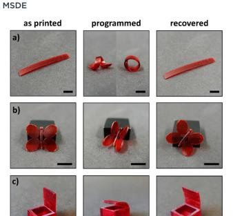
Fig. 4 Shape memory test of DLP-printed structures. Initial (as printed), temporary and recovered shape of a) strip, b) butterfly, c) box. Programming was performed in hot water at 95 °C, followed by fixation in cold water at 15 °C. Successive shape memory recovery was initiated by blue laser light irradiation (450-460 nm) at 567 mW cm<sup>-2</sup>. Scale bar = 10 mm.
