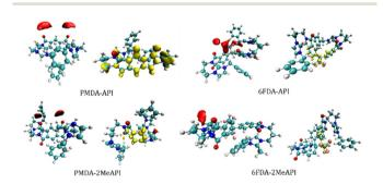
Fig. 11 The SDFs of anions (red) and cationic polymer chains (gold) around the positively charged polymer chain. The corresponding isovalues for the anion and cationic species of number densities are 10 nm<sup>-3</sup> and 4 nm<sup>-3</sup>, respectively. The central positively charged polymer chain are represented as CPK models.
