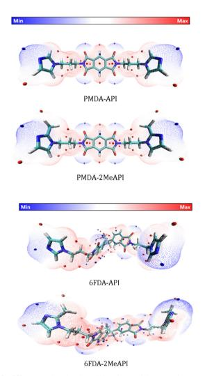
Fig. 9 ESP-mapped molecular vdW surfaces of the neutral monomers, corresponding to the  $\rho=0.001$  e/Bohr³ isosurface. The color scale bar is shown at the top, while the corresponding ESP values (units of kcal  $\rm mol^{-1})$  are -50-50 kcal  $\rm mol^{-1}$ . The local minima and maxima points on the ESP surface are represented as blue and red spheres, respectively. These species are represented as licorice models (cyan: C, white: H, red: O, blue: N, and pink: F).
