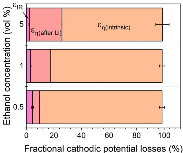
Fig. 4 A plot to show the fractional potential losses in the cathodic reaction for the lithium-mediated nitrogen reduction system due to overpotential and ohmic losses for a 0.6 M  $\text{LiClO}_4$  in THF electrolyte with varying ethanol content. Fractional energy losses obtained using eqn (18) and (19).
