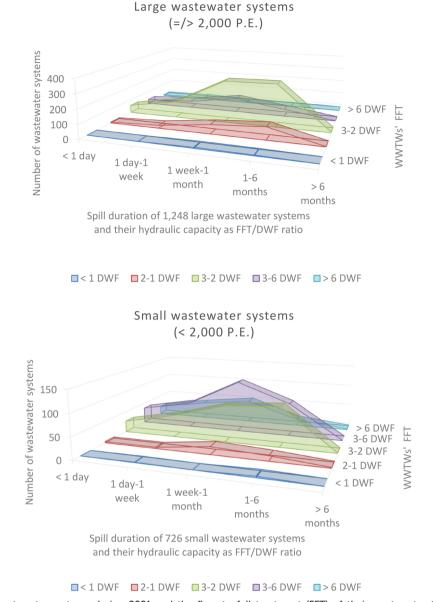
Fig. 3 Spill duration of wastewater systems during 2021 and the flow to full treatment (FFT) of their wastewater treatment works (WWTWs) expressed as multiples of dry weather flow (DWF) in five categories: spilled up to a day (=/<1 d); spilled between a day and a week (1 d-1 w); spilled between a week and 1 month (1 w-1 m); spilled between 1 and 6 months (1 m-6 m); and spilled more than 6 months (>6 m).
