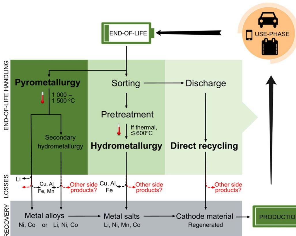
Fig. 3 Overview of handling, material losses, and material recovery for the three major LIB recycling processes: pyrometallurgy, hydrometallurgy and direct recycling. Temperatures are  $\cong$  ambient when not stated. Dashed arrows indicate fractions that are not possible to recycle using a given process. Figure adapted from Kushnir, 2015<sup>86</sup> and Lv *et al.*, 2018.<sup>85</sup>
