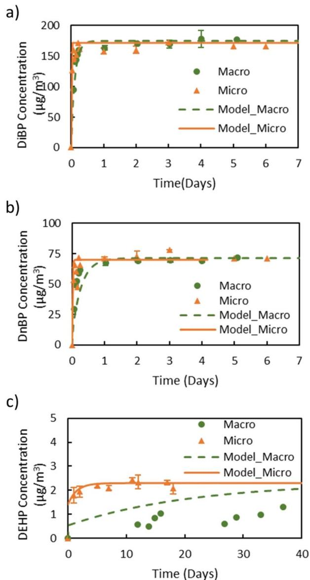
Fig. 2 Comparison of the gas-phase concentrations of selected plasticizers over time in the macro chamber and in the micro chamber for (a) DiBP, (b) *Dn*BP, and (c) DEHP. Dots and triangles refer to measured gas-phase concentrations in the macro and micro chamber, respectively, while the lines are DustEx model predictions.
