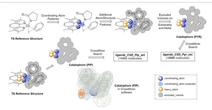
Fig. 3 Workflow for generation of a catalophore from a transition state reference structure and identification ligands in the CSD to generate ligand sets ligands\_CSD\_Pip\_set and ligands\_CSD\_Pyr\_set. Hydrogens are excluded for clarity.
