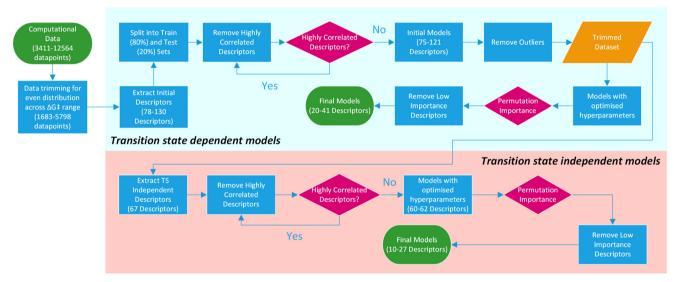
Fig. 9 Overview of the machine learning model generation process, from computational data to final models.
