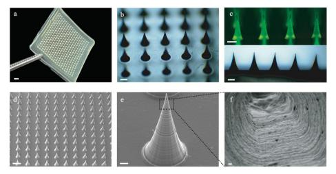
Fig. 2 Apparent characterization of HMNs. (a) Optical image of HMNs; scale bar: 2 mm. (b) Optical microscopy images of HMNs, 4x; scale bar: 200  $\mu$ m. (c) Fluorescence microscopy images of calcein-loaded HMNs (up, 5x) and optical microscopy images of HMNs (down, 4x); scale bar: 200  $\mu$ m. (d and e) SEM images of HMNs. Scale bar in (d), 500  $\mu$ m; scale bar in (e), 50  $\mu$ m. (f) SEM image of the lyophilized HMNs showing the porous structure; scale bar: 2  $\mu$ m.
