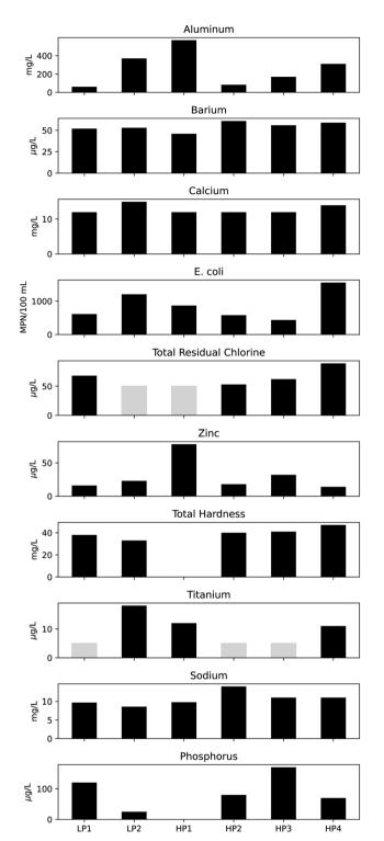
Fig. 7 Results from analysis of samples collected with the automatic sampler (light gray bars reflect samples below detection limit).
