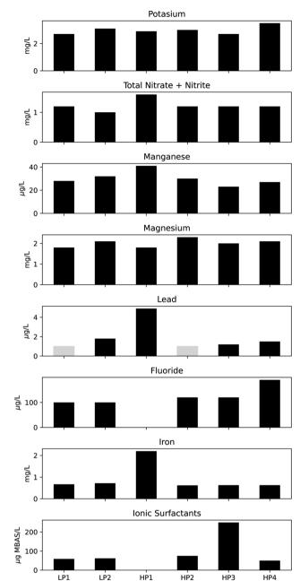
Fig. 8 Additional results from analysis of samples collected with the automatic sampler (light gray bars reflect samples below detection limit).
