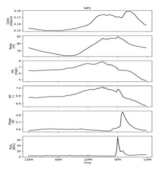
Fig. 11 Sensor signals during day of sample HP1. High probability sampling event corresponded to an alarm at 4:09 PM related to the specific conductivity signal.
