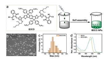
**Fig. 1** (a) The molecular structure of IEICO and the preparation of IEICO NPs. (b) SEM image. (c) Particle size distribution histograms of IEICO NPs. (d) The normalized absorbance spectrum of IEICO in THF and IEICO NPs in water.
