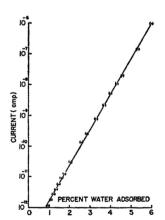
Fig. 2 Conductivity/current of crystalline bovine haemoglobin as a function of water content at room temperature. Reprinted from B. Rosenberg, J. Chem. Phys., 1962, 36, 816-823, with the permission of AIP Publishing. 16
