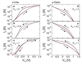
Fig. 13 The transfer characteristics for transistors based upon semiconductor nanowires and a PEO top gate (wire type indicated).  $P_{\text{rel}}$ indicates the relative water vapour pressure (i.e. relative humidity). Reprinted with permission from D. J. Carrad et al. Nano Lett., 2017, 17, 827-833. Copyright 2017 American Chemical Society.81
