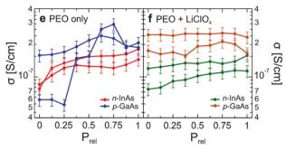
Fig. 14 Conductivity of the PEO top gate as a function of relative pressure (relative humidity) using the nanowire transistors in Fig. 12 and 13. Doping with/without LiCl is indicated. D. J. Carrad *et al. Nano Lett.*, 2017, **17**, 827–833. Copyright 2017 American Chemical Society.<sup>81</sup>
