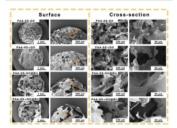
**Fig. 3** The representative surface and cross-sectional SEM images of the PAA-SS-GO, PAA-SS-rGO, PAA-SS-GO@BIL and PAA-SS-rGO@BIL beads. The typical gel porous channel structures are marked by orange arrows.
