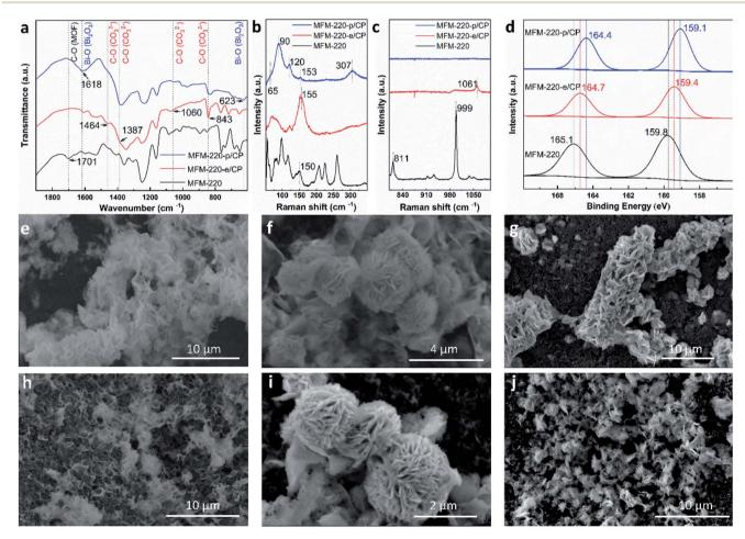
Fig. 2 Characterisation of the transformation and evolution of Bi-MOFs to  $Bi_2O_2CO_3$  nanosheets and  $\alpha$ - $Bi_2O_3$ . (a) FT-IR spectra; (b and c) Raman spectra; (d) XPS spectra; SEM images of (e) MFM-220-e/CP, (f) MFM-221-e/CP, (g) MFM-222-e/CP, (h) MFM-220-p/CP, (i) MFM-221-p/CP, and (j) MFM-222-p/CP.
