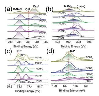
Fig. 2 High resolution XPS spectra of the (a) C 1s, (b) N 1s, (c) Pt 4f, and (d) P 2p electrons of the PtCN, PtCNP<sub>1</sub>, PtCNP<sub>2</sub>, PtCNP<sub>3</sub>, and PtCNP<sub>4</sub> samples.
