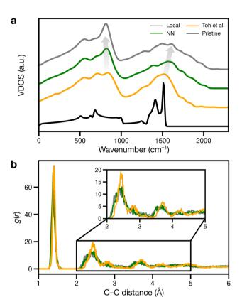
**Fig. 6** Signatures of structural disorder. (a) Vibrational density of states (VDOS) for the different structures and pristine graphene (black line). The gray arrows indicate trends in peak shifts. (b) Radial distribution functions, *g*(*r*), for the different structures.
