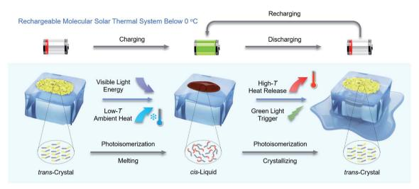
Fig. 1 Schematic representation of a rechargeable molecular solar thermal system below 0 °C, which stores energy from both visible light energy and low-temperature ambient heat, and then discharges it on demand in the form of high-temperature heat.
