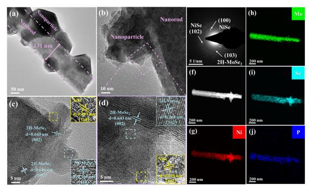
Fig. 2 (a and b) TEM images, (c and d) HRTEM images, (e) SAED image, and (f-j) elemental mapping of P-NiSe/MoSe<sub>2</sub>@NF.
