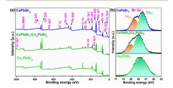
Fig. 3 (a) Wide-scan X-ray photoelectron spectrum of emissive CsPbBr<sub>3</sub>, dual-phase CsPbBr<sub>3</sub>/Cs<sub>4</sub>PbBr<sub>6</sub> and non-emissive Cs<sub>4</sub>PbBr<sub>6</sub>. (b) High-resolution X-ray photoelectron spectra of Br (3d).
