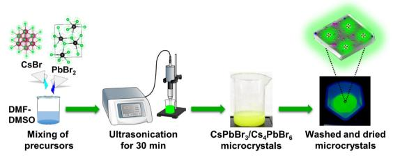
Fig. 1 Scheme for the synthesis of dual-phase CsPbBr<sub>3</sub>/Cs<sub>4</sub>PbBr<sub>6</sub> MCs using ultrasonication process.
