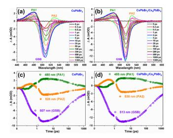
Fig. 6 Femtosecond transient absorption (fs-TA) spectra of (a) CsPbBr<sub>3</sub>, (b) CsPbBr<sub>z</sub>/Cs<sub>4</sub>PbBr<sub>c</sub> measured for various pump-probe delay times at 400 nm excitation, excited-state kinetic curves for the PA1, GSB, and PA2 of (c) CsPbBr<sub>3</sub>, (d) CsPbBr<sub>3</sub>/Cs<sub>4</sub>PbBr<sub>6</sub>
