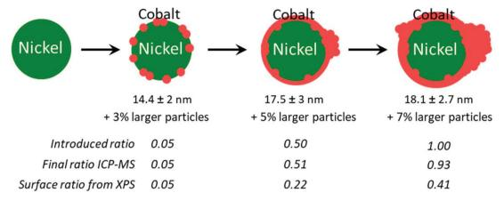
Fig. 9 Proposed mechanism for the cobalt reaction with the nickel nanoparticles at selected stages. The bottom table recalls selected Co/Ni ratio. The top values recall the average diameters of the smaller NP population as well as the amount of larger NPs.
