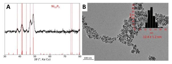
Fig. 1 (A) XRD pattern of the nanoparticles powder, the reference phase in red corresponds to Ni<sub>12</sub>P<sub>5</sub> (PDF 03-065-4018, dotted lines are a guide to the eye). (B) TEM of the nanoparticles and size distribution in the inset.
