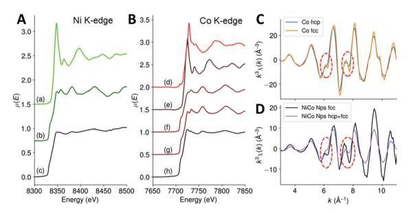
Fig. 3 (A) XANES of the fcc NiCo NPs at Ni K-edge, (a) NiO ref, (b) Ni(0) foil ref, (c) NiCo NPs. (B) XANES of the fcc NiCo NPs at Co K-edge, (d)  $Co_3O_4$  ref, (e) CoO ref, (f) Co(0) hcp ref, (g) Co(0) fcc ref<sup>40</sup> and (h) NiCo NPs. (C and D) EXAFS at Co K-edge of (blue) Co hcp, (orange) Co fcc, (black) fcc NiCo NPs and (violet) fcc + hcp NiCo NPs. The red circles are a guide to the eye to point the features used to discriminate between Co hcp and fcc phases.
