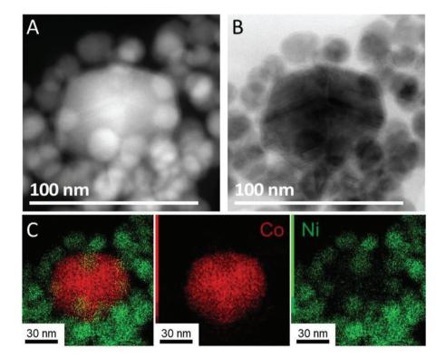
Fig. 5 (A) STEM-HAADF, (B) STEM bright field and (C) STEM-EDS mapping of NiCo NPs synthetized using 1 equiv. of TOP and temperature steps (red for cobalt and green for nickel).
