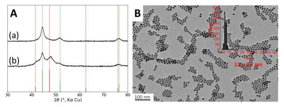
Fig. 2 (A) XRD pattern of two samples (a and b) prepared in diluted conditions, the reference phase in green corresponds to *fcc* Ni (JCPDS file 00-004-0850) and the reference phase in red corresponds to *hcp* cobalt (JCPDS file 04-001-3273). (B) Representative TEM of the nanoparticles and size distribution in the inset.
