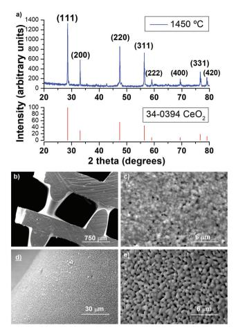
Fig. 3 XRD pattern of the ceria scaffold sintered at 1450  $^{\circ}$ C, with the major peaks for cubic CeO<sub>2</sub> indexed. SEM images of a sintered and polished scaffold (b) show the interior (c) and exterior (d–e) microstructure.
