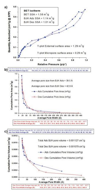
Fig. 4 BET isotherm (a) and BJH cumulative pore area (b) and pore volume (c) plots for N<sub>2</sub> adsorption/desorption on sintered ceria scaffolds. The boxes show the pore width range intervals and pore width average data point values for adsorption (blue) and desorption (red).
