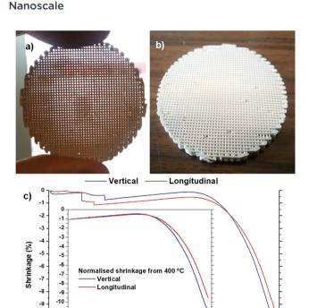
Fig. 2 Photographs of the sintered robocast ceria scaffolds (a–b), and their shrinkage in the vertical and longitudinal directions with heating (c).
