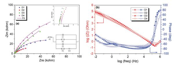
Fig. 8 Electrochemical impedance spectra of the asymmetric supercapacitors D1, D2, D3 and D4 with a 6 M KOH electrolyte. (a) Nyquist plot (top inset: high frequency region and bottom inset: equivalent circuit used to fit the experimental data) and (b) Bode plot.
