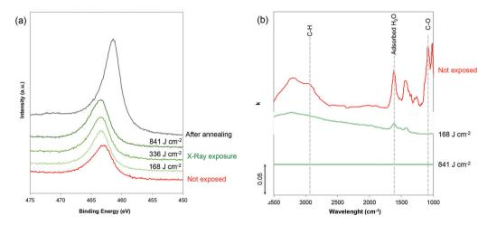
Fig. 2 (a) XPS spectra recorded in the Ru(3p) region on films exposed to different doses and annealed under a reducing atmosphere. (b) Evolution of the extinction coefficient k of a RuCl<sub>3</sub>/F127 film before and after exposure at different doses.
