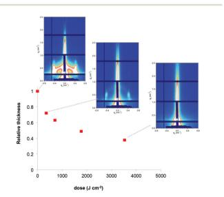
Fig. 3 Evolution of the relative thickness of the RhCl<sub>3</sub>/F127 films as a function of X-ray dose. Inset: the corresponding GISAXS patterns.
