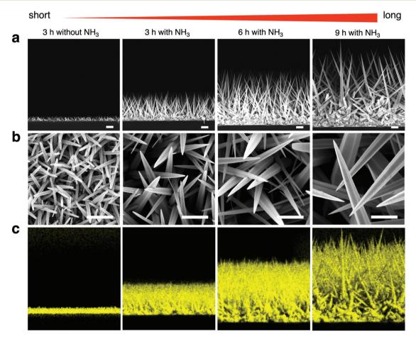
Fig. 1 (a) FESEM images of cross-sectional nanowires for different growth conditions. The scale bars are 2 μm. (b) FESEM images of top-view nanowires. The scale bars are 1  $\mu$ m. (c) Elemental mapping of Zn K $\alpha$  (8.6313 keV) highlighted in yellow, as a main constituent of the nanowires.
