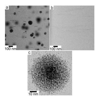
Fig. 3 LPTEM and dry HRTEM images indicate supraparticles formed by assembly of 2 nm primary particles formed in bulk solution. (a) and (b) Bright field LP-TEM images showing horizontal steaks in (a) 1 M TBA (pixel dwell time of 25  $\mu s$  and frame rate of 0.04 frames per s) and (b) 1 M TBA and 1 mM SC (pixel dwell time of 5  $\mu s$  and frame rate of 0.2 frames per s). (c) Dry state HRTEM image showing free platinum primary particles attached to the substrate near a supraparticle.
