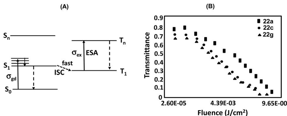
Fig. 17 (A) Proposed energy-level model depicting photophysical processes (ISC: intersystem crossing, ESA: excited state absorption leading to RSA); (B) normalized transmittance of **22a**, **22c** and **22g** as a function of the fluence of laser pulse (527 nm). Reproduced with permission from ref. 39. Copyright 2016, The Royal Society of Chemistry.
