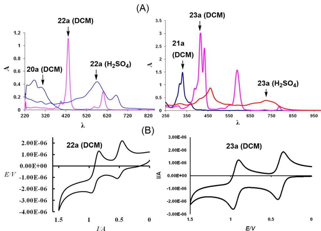
Fig. 2 (A) UV-visible absorption spectra (**20a/22a** in DCM and  $\text{H}_2\text{SO}_4$ ; **21a/23a** in DCM) and (B) cyclic voltammograms of **22a** and **23a** (DCM, electrolyte:  $\text{TBAPF}_6$ ; working electrode: Pt; reference electrode:  $\text{Ag}/\text{AgCl}$ ;  $80 \text{ mV s}^{-1}$ ). Reproduced with permission from ref. 13 and 14. Copyright 2011 and 2012, respectively, The Royal Society of Chemistry.
