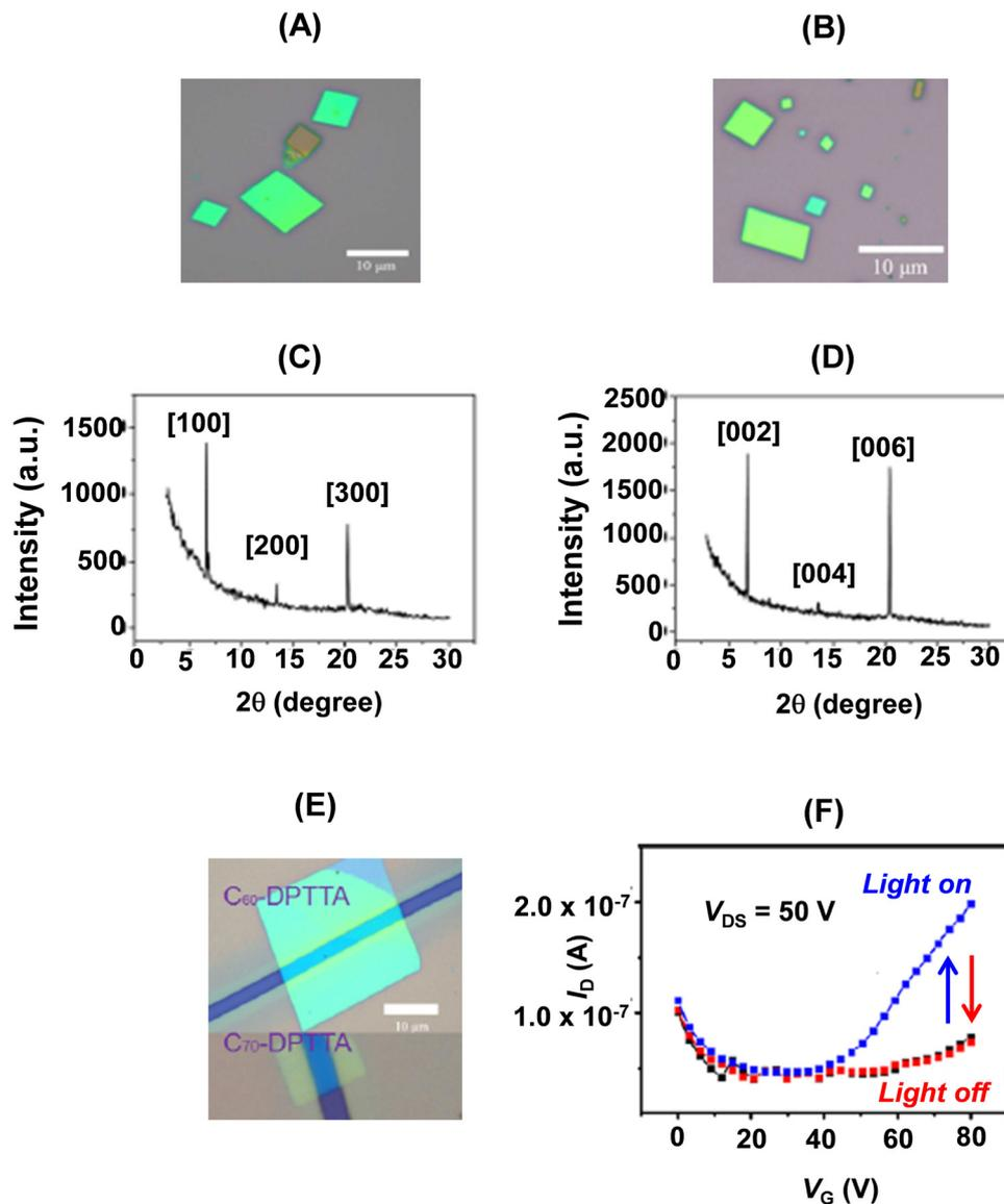
Fig. 15 Optical micrographs of self-assembled **22a**-C<sub>60</sub> (A) and **22a**-C<sub>70</sub> (B); XRD patterns of **22a**-C<sub>60</sub> (C) and **22a**-C<sub>70</sub> (D); (E) optical image of the single crystal BGTC devices; (F) photocurrent responses of the **22a**-C<sub>70</sub> microcrystal based transistor under light irradiation. Reproduced with permission from ref. 32. Copyright 2013, The American Chemical Society.
