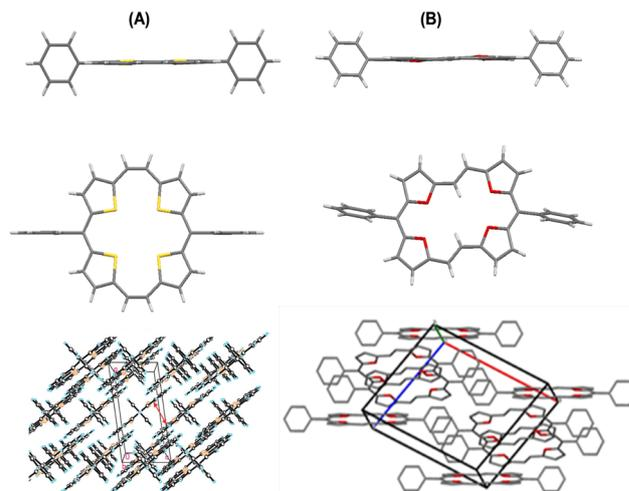
Fig. 3 Single crystal X-ray structures: side views, top views and stacking patterns of **22a** (A) and **23a** (B). Reproduced with permission from ref. 13 and 14. Copyright 2011 and 2012, respectively, The Royal Society of Chemistry.
