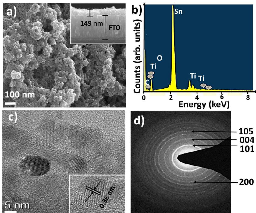
Fig. 3 (a) FESEM plan-view image, (b) EDX pattern, (c) HR-TEM image, and (d) SAED pattern of SILAR-grown  $\text{TiO}_2$  film. Adapted with permission from ref. 23. Copyright (2018), Springer Nature Research.
