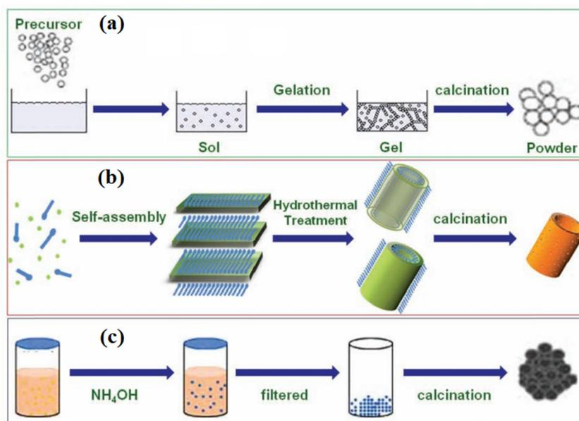
**Fig. 2** A schematic representation of the chemical synthesis of MONs employing different processing methods, *i.e.*, (a) sol-gel, (b) hydrothermal, and (c) co-precipitation. Adapted from ref. 21. Copyright (2017), Royal Society of Chemistry.
