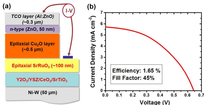
Fig. 4 (a) Device design and (b) current–voltage characteristics of a flexible solar cell, which has an epitaxial Cu<sub>2</sub>O absorber-layer on the textured metallic substrate. Adapted from ref. 41, Copyright (2015), Springer Nature Research.
