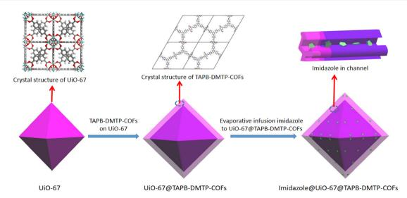
Scheme 1 Schematic of the synthetic route to imidazole@UiO-67@TAPB-DMTP-COFs.
