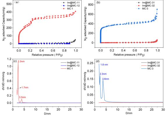
Fig. 3 N<sub>2</sub> adsorption-desorption isotherms (a and b) and pore-size distributions (c and d) of the samples.
