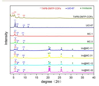
Fig. 1 PXRD patterns of the samples.
